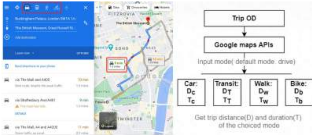
Fig. 2. The process of crawling potential substituted mode information from the Google Map developers API. (The base map is from Google map)
